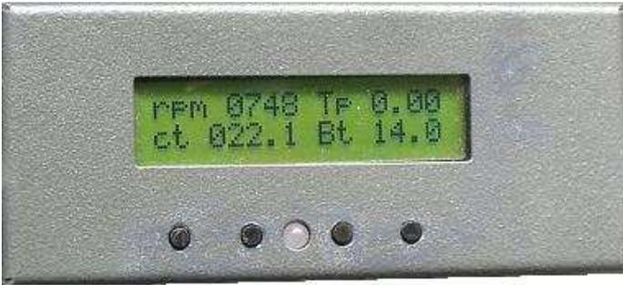
In this working mode the NANOCOM starts automatically to read and shows the four main fuelling parameters with the frequency of four times per second as a board's instrument. The Nanocom turns itself to standby a few seconds after you turn off the ignition.
